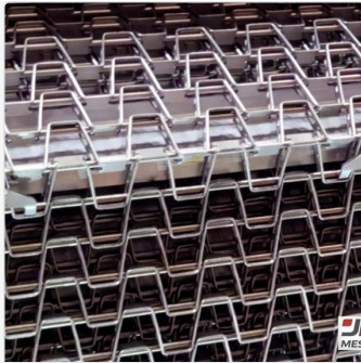
Lift plates fitted Height and spacing per drawing
