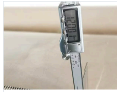
Side plate height checked: 120 mm
