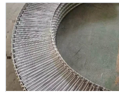
Belt laid out on a curve
