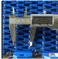
POM mesh · rod pitch 31.75 mm
