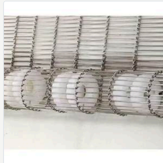
UHMWPE sprockets on the shaft
